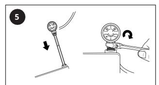
Slowly insert the element into the inlet at an angle to avoid spillage. With an adjustable spanner turn clockwise to tighten the element into the radiator inlet. **DO NOT** twist the head by hand as this can damage the element beyond repair.
