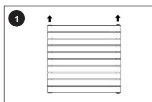
Unbox and stand your radiator with the inlet(s) you will be inserting the element into facing upwards, it is advised to place the radiator on a protective sheet due to potential spillage.
