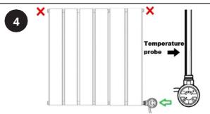
If the temperature probe is positioned on the left side when the element is front facing, the element will need to be installed on the right inlet to allow for the probe to be positioned at the bottom as referenced in step 2. \*This will be the opposite if the temperature probe is positioned on the right side of the front facing element.
