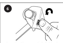
With an adjustable spanner, check all of the inlet/outlet blanking plugs to ensure that they are all secure to avoid any glycol leakage before switching the radiator on. Please take care not to over tighten the blanking plugs.
