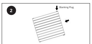
With the radiator still on the protective sheet, position the radiator at an angle and remove the top blanking plug. This will allow you to insert the element into the radiator without losing any glycol and also allow you to check the glycol level is correct. \*Please see step 1 of the "temperature issues" for reference on correct glycol levels.
