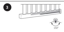
When the element is installed horizontally, the temperature sensor (single probe) must be positioned as low as possible in the bottom collector bar to get the best possible heat output. \*Please note, the position of the temperature probe is not fixed and may differ. This can determine which side inlet (left/right) the element is fitted to in order for the element face to be front facing. See step 4 of "Installation advice" for an example of probe positioning.
